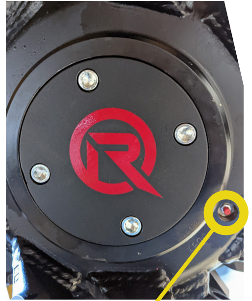
Grease port on the drum
