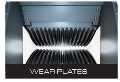
ROCKCRUSHER has replaceable cheek plates to help avoid wear on the frame structure.
