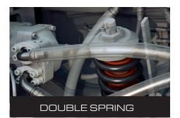
ROCKCRUSHER's double spring system reduces the potential for spring malfunction while stabilizing the toggle plate and buffering the movement of the jaw plates.
